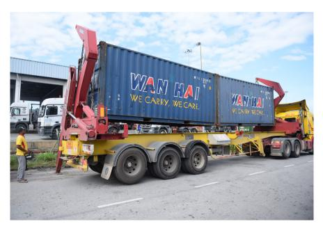
taking shape for the family owned logistics company. The Company found its niche, and has steadily scaled its business by expanding its fleet of prime movers and recently taking delivery of two new Steelbro SB450 sidelifters.
